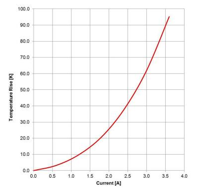
DESCRIPTION Projection **WE-LHMI SMD Power Inductor** Würth Elektronik eiSos GmbH & Co. KG EMC & Inductive Solutions Max-Eyth-Str. 1 Order.- No. 1.2 2012-06-28 SSt SSt 74638 Waldenburg COMPLIANT SIZE Germany RoHS&REACh 1.1 2012-02-29 SSt BD Tel. +49 (0) 79 42 945 - 0 WÜRTH ELEKTRONIK 74437324033 www.we-online.com A4 1.0 SSt 2011-10-01 BD eiSos@we-online.com REV DATE ΒY CHECKED Size: 4020
